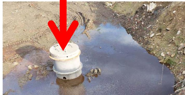
**Same puddle after the injections – Cr<sup>6+</sup> was reduced and later precipitated causing a color change**
